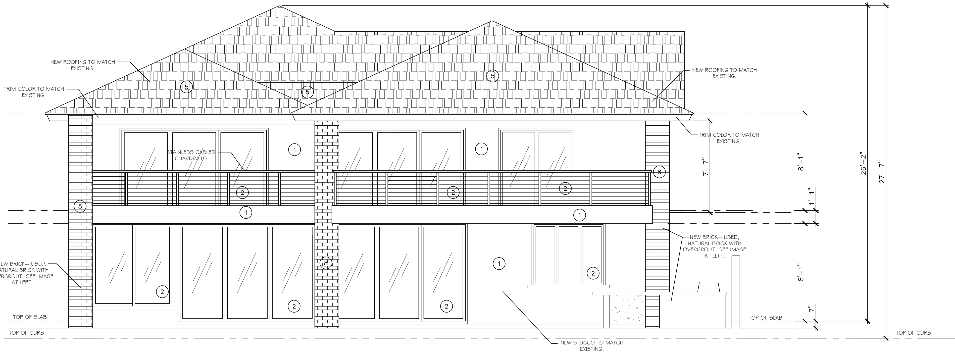
PROPOSED REAR ELEVATION
