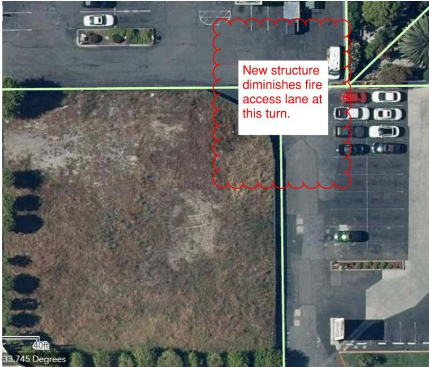
**Hose Pull Lengths** – The fire apparatus access road shall comply with the requirements of Section 503.1.1 of the Huntington Beach Fire Code. All access roads shall extend to within 150 feet of all portions of the exterior walls of the first story of the building as measured by an approved route around the exterior of the building or facility.
