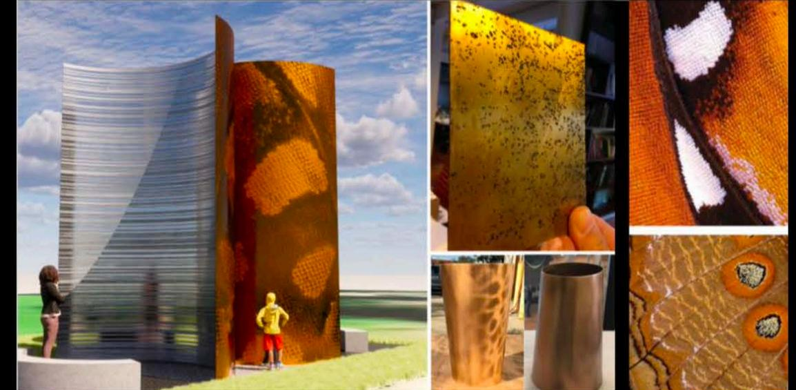
VARIETY OF TEXTURED SURFACE THROUGH CNC BEAD ROLLING OR MECHANICAL "DUMPLE" DEFORMATION IT
