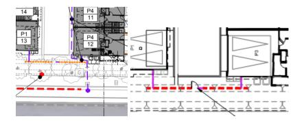
*Fire Access Road Turns and Corners* shall be designed with a minimum inner radius of seventeen feet (17') and a minimum outer radius of forty five feet (45') per City Specification # 401 *Minimum Standards for Fire Apparatus Access*. For Fire Department approval, reference and demonstrate compliance with City Specification # 401 *Minimum Standards for Fire Apparatus Access* on the plans. **(FD)**
