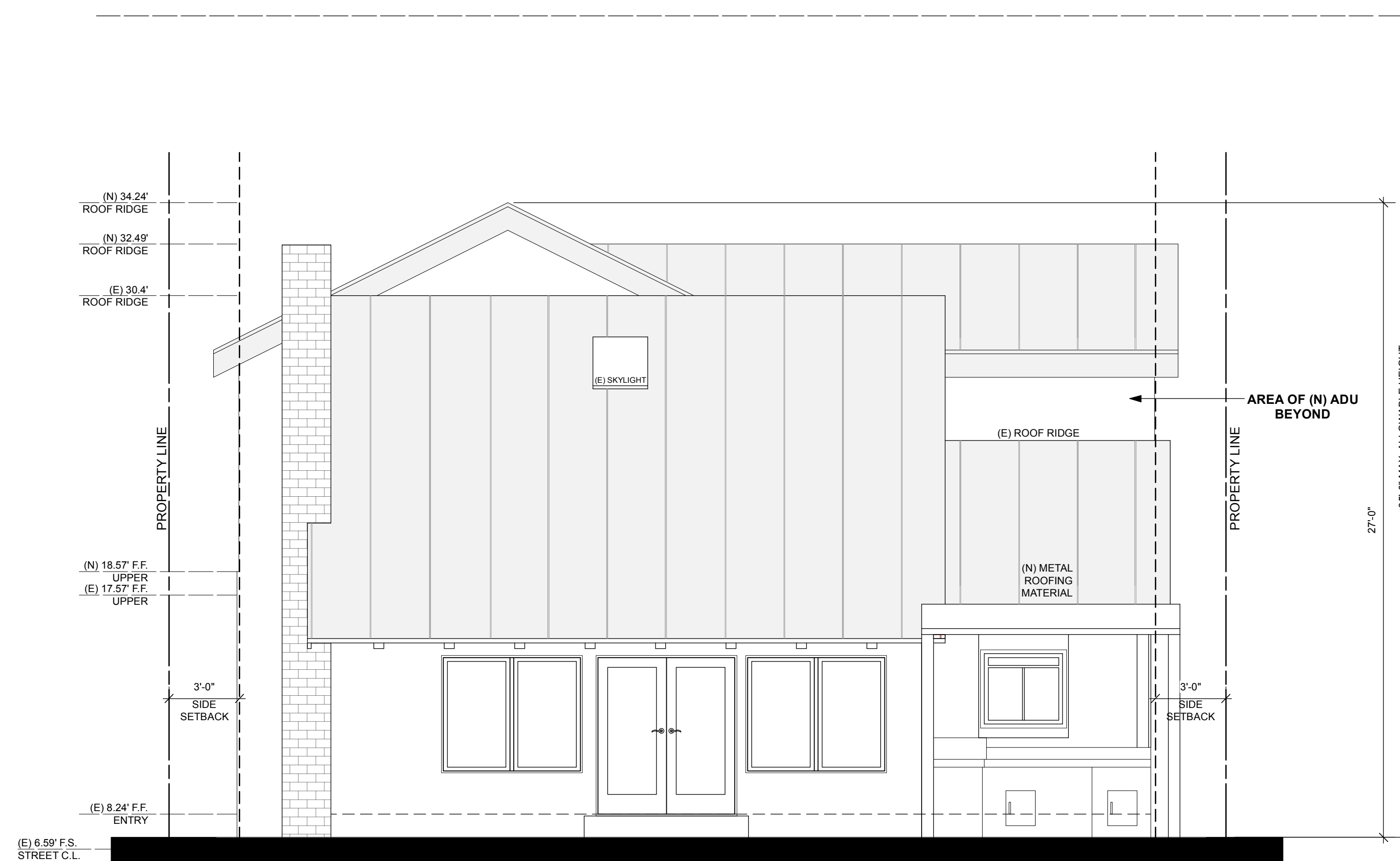
PROPOSED REAR / SOUTH-WEST ELEVATION 1/4"=1'-0"
