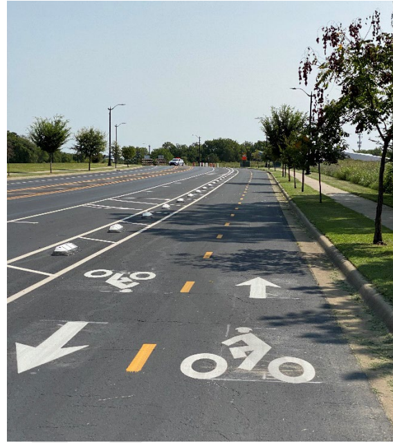
Figure 13: Class IV – Two-Way Separated Bikeway (Outside of Huntington Beach)
