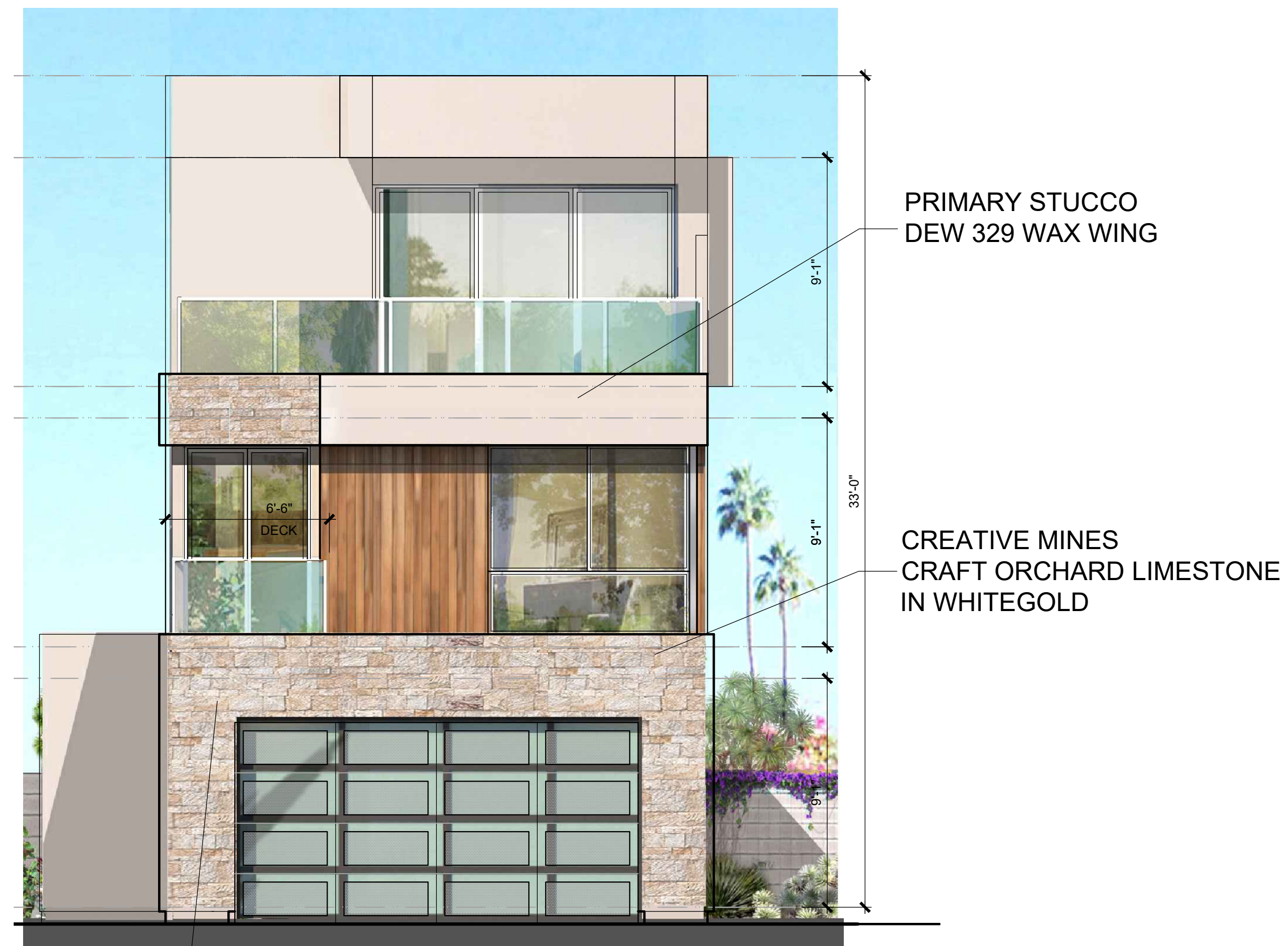
FRONT ELEVATION MANUF. VENEER CRAFT ORCHARD LIMESTONE MAX. HEIGHT 35'
