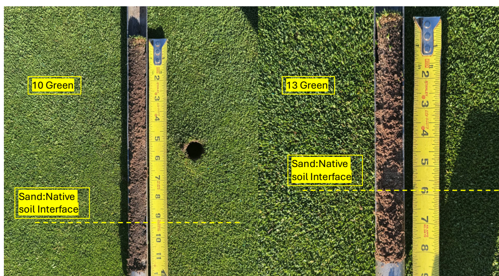
The improved profile with sand and organic matter is deep on No. 10 green (left) at 9 inches but much shallower on No. 13 green (right) at about 6 inches.
