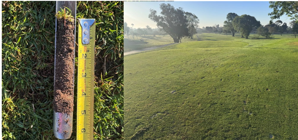
The rootzone in tees is comprised of about 5 inches of sand and organic material on top of the native soil (No. 10 tee rootzone and tee surface shown here).
