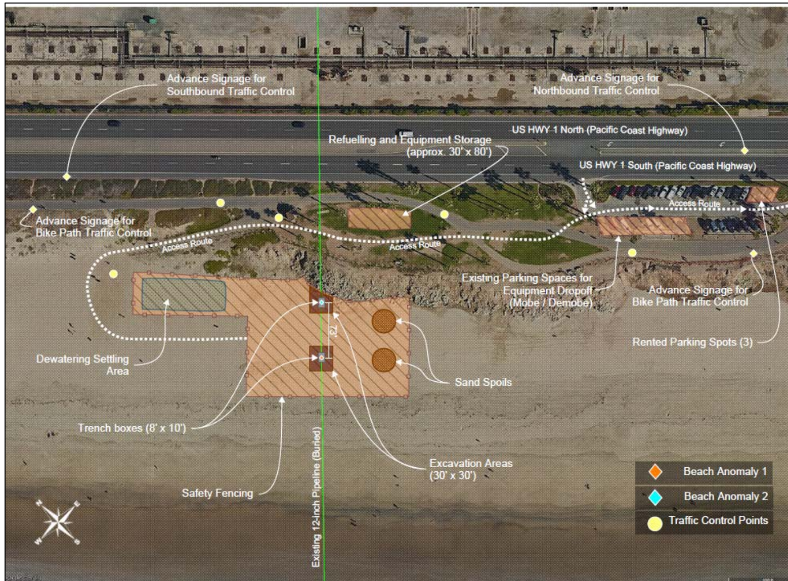
Figure 1.1-2. Site Plan View
