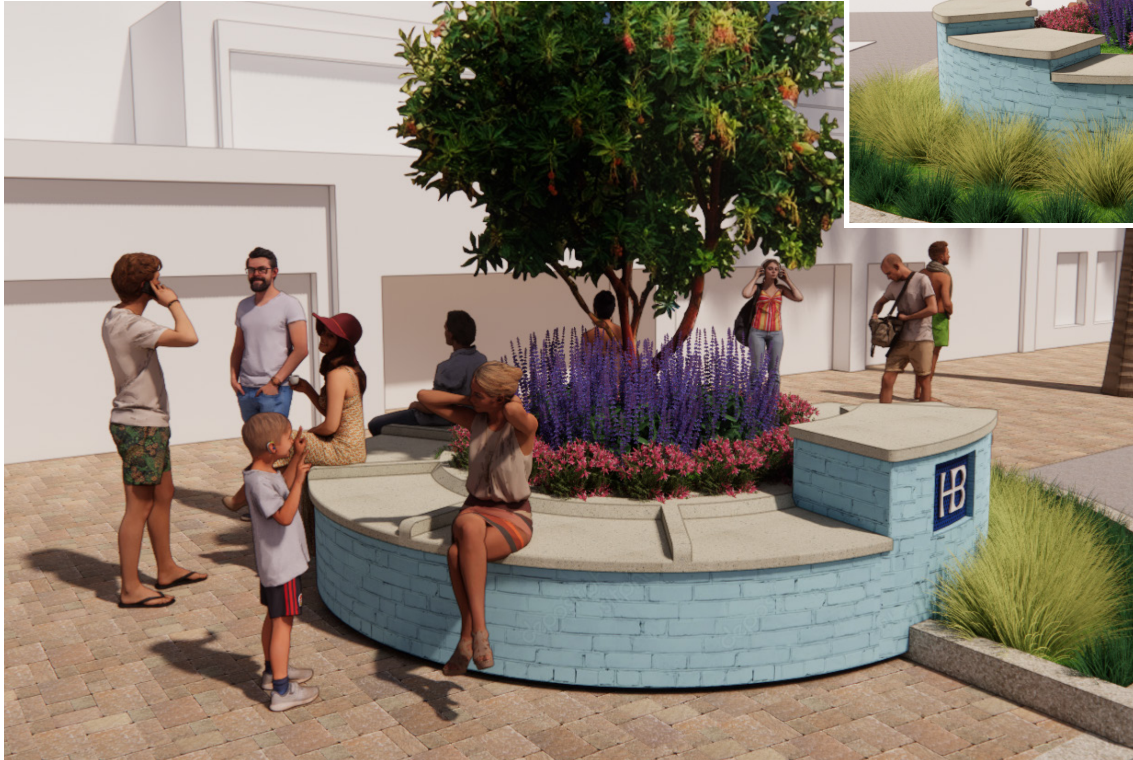
Pre-cast concrete wall cap in sand color with acid etch texture
