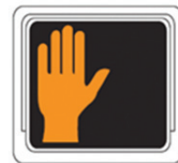
Figure 5. A flashing upraised hand signal indicates to the pedestrian "DON'T WALK" or do not enter the roadway.
