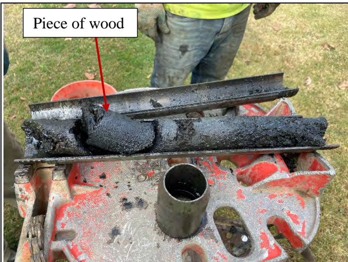
First split spoon sample collected at 30 – 31.5 ft bgs at HSA-5. Sample indicates of the presence of waste.
