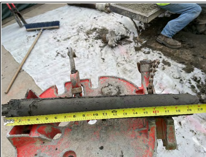
Split spoon sample collected at 10 – 11.5 ft bgs at HSA-5A.
