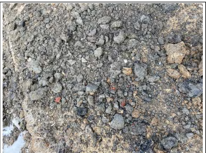
Brick pieces observed in the drill cuttings at HSA-4A
