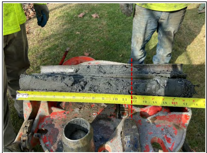
Split spoon sample collected at 40 – 41.5 ft bgs at HSA-5. The interface between the waste and native soil is indicated.
