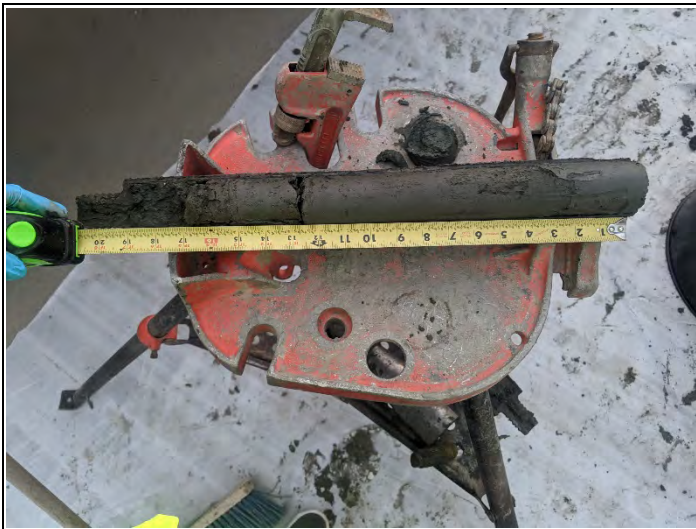
Split spoon sample collected at 10 – 11.5 ft bgs at HSA-6A.
