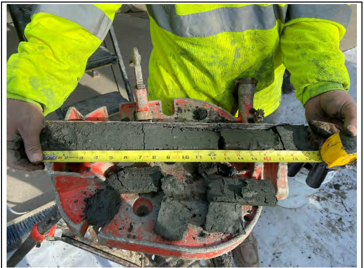
Split spoon sample collected at 15 – 16.5 ft bgs at HSA-4A.
