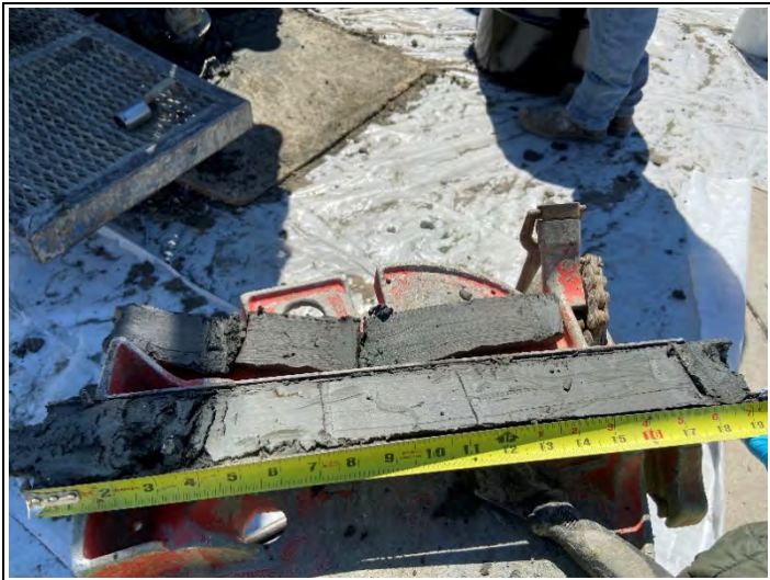
Split spoon sample collected at 10 – 11.5 ft bgs at HSA-3A.
