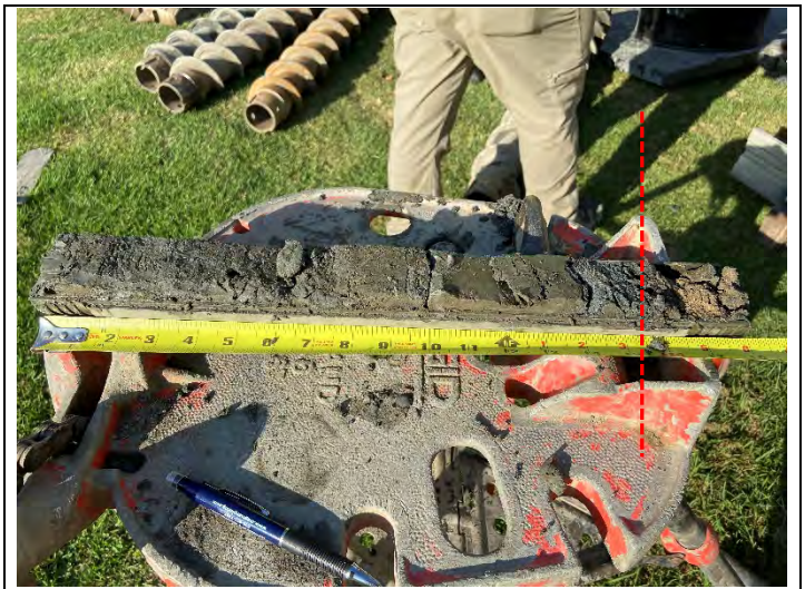
Split spoon sample collected at 10 – 11.5 ft bgs at HSA-1. The interface between the waste and native soil is indicated.
