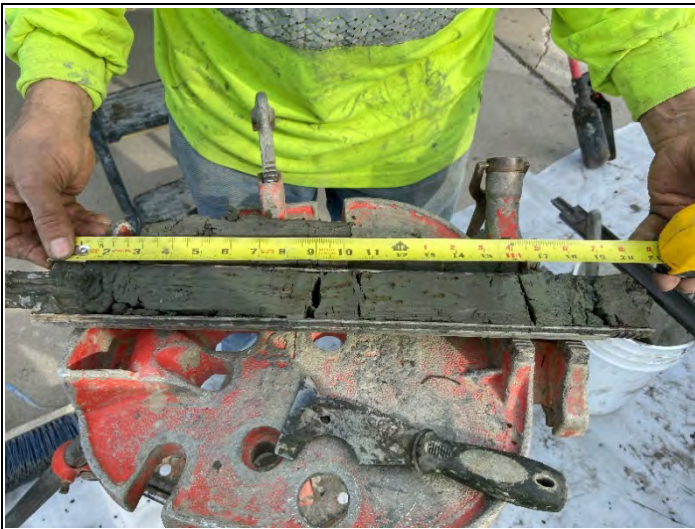
Split spoon sample collected at 10 – 11.5 ft bgs at HSA-4A.
