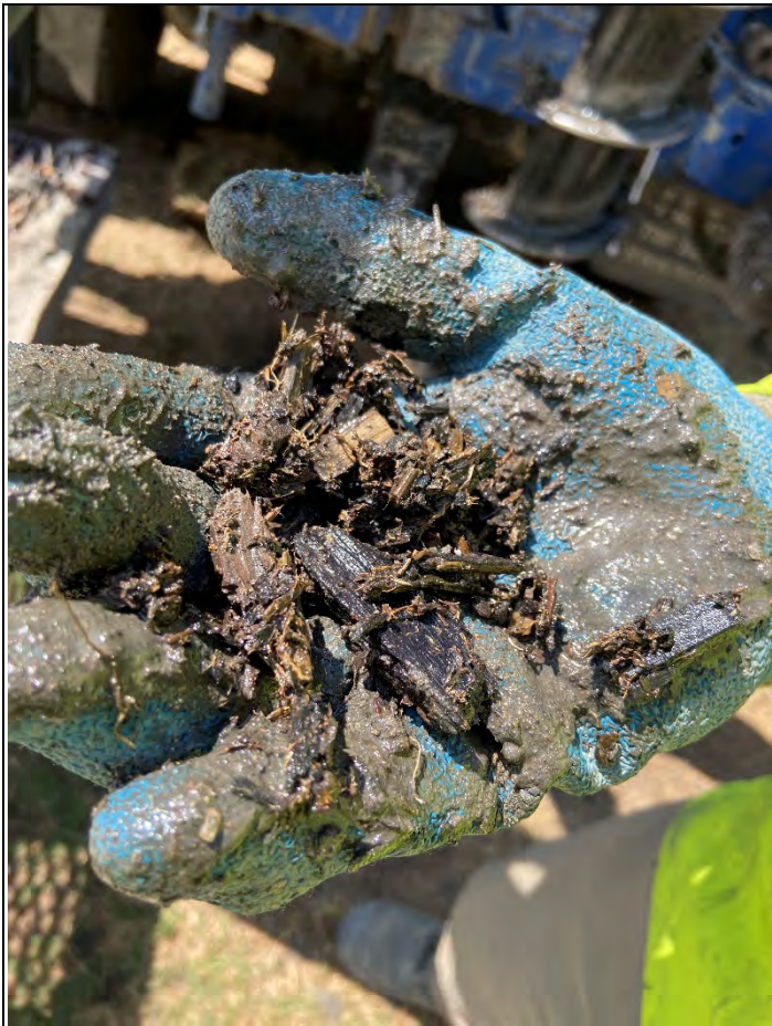
Spoil (wood debris) retrieved from the auger at HSA-4.
