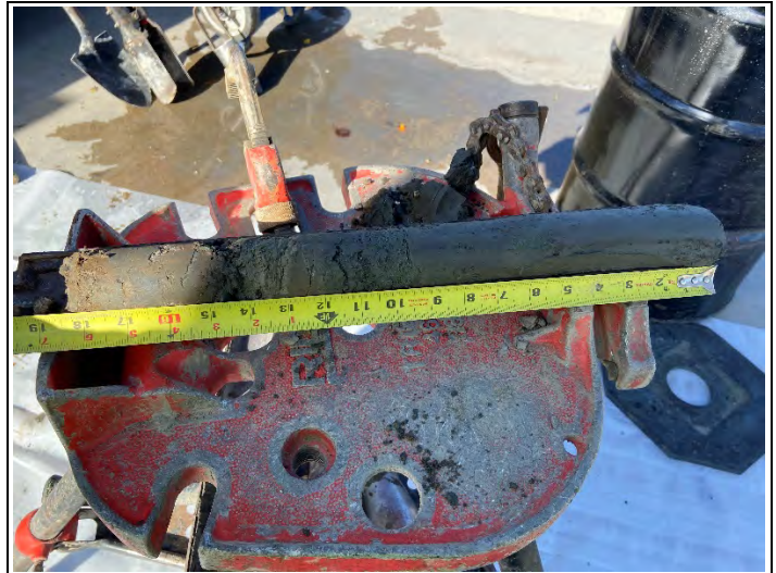
Split spoon sample collected at 10 – 11.5 ft bgs at HSA-7A.
