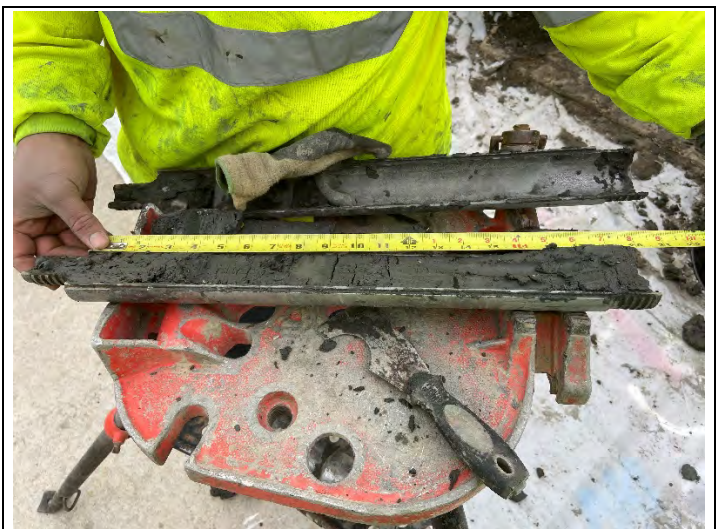
Split spoon sample collected at 15 – 16.5 ft bgs at HSA-5A.
