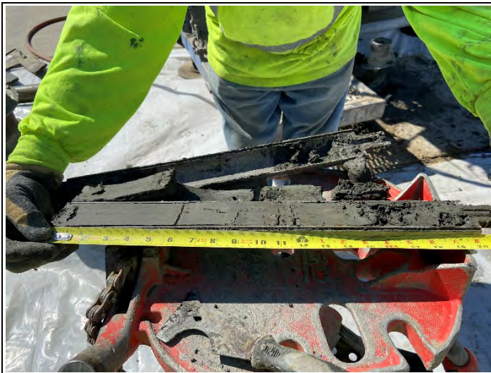
Split spoon sample collected at 10 – 11.5 ft bgs at HSA-2A.
