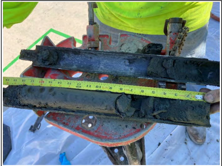
Split spoon sample collected at 10 – 11.5 ft bgs at HSA-8A.
