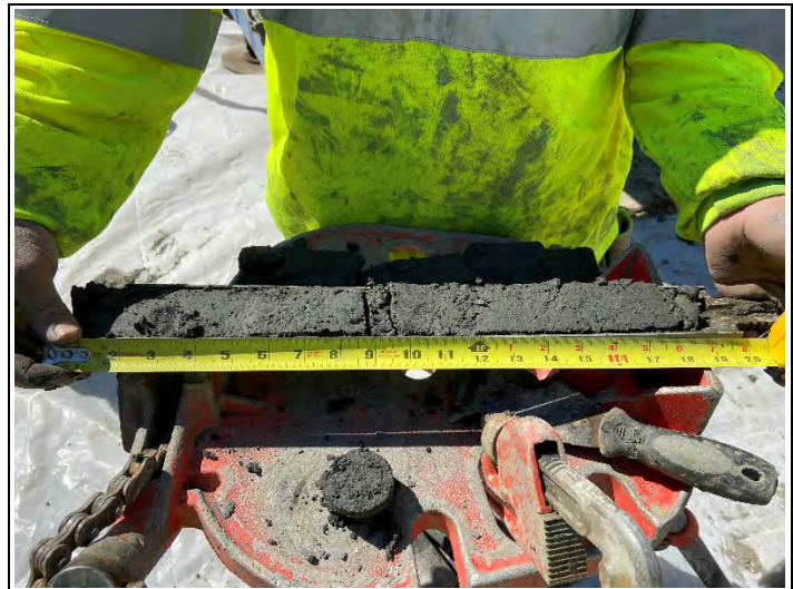
Split spoon sample collected at 15 – 16.5 ft bgs at HSA-2A.
