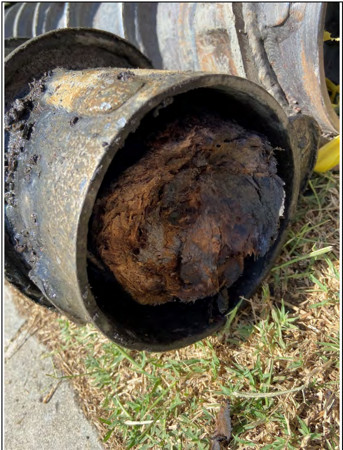
Wood plugged in the lead auger at HSA-4.
