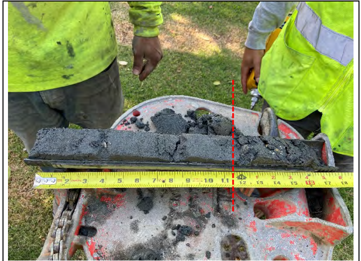
Split spoon sample collected at 15 – 16.5 ft bgs at HSA-2. The interface between the waste and native soil is indicated.
