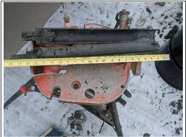
Split spoon sample collected at 15 – 16.5 ft bgs at HSA-6A.
