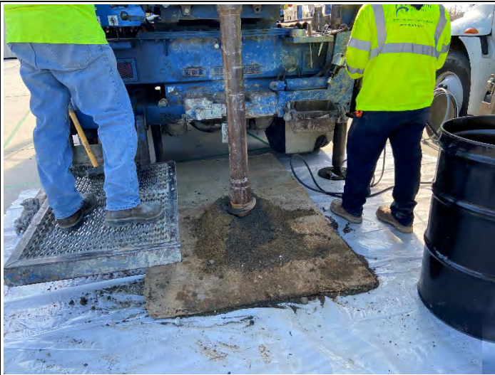
Change in material observed in the drill cuttings at HSA-7A (looking east)
