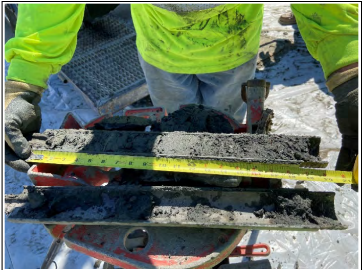
Split spoon sample collected at 15 – 16.5 ft bgs at HSA-3A.
