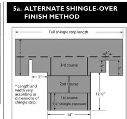
1. TRIM two shingle strips to lengths shown for Courses 1 and 2. Using a full length of shingle strip, trim to pattern dimensions shown for Course 3.
