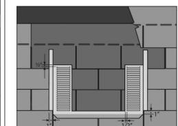
2. BEGINNING WITH COURSE 1, align and attach to top of vent as shown using locally-approved peel and stick, two-sided tape, or sealant (Class A where required by code for flame resistance). Repeat with Courses 2 and 3 to complete shingle-over finish method.
