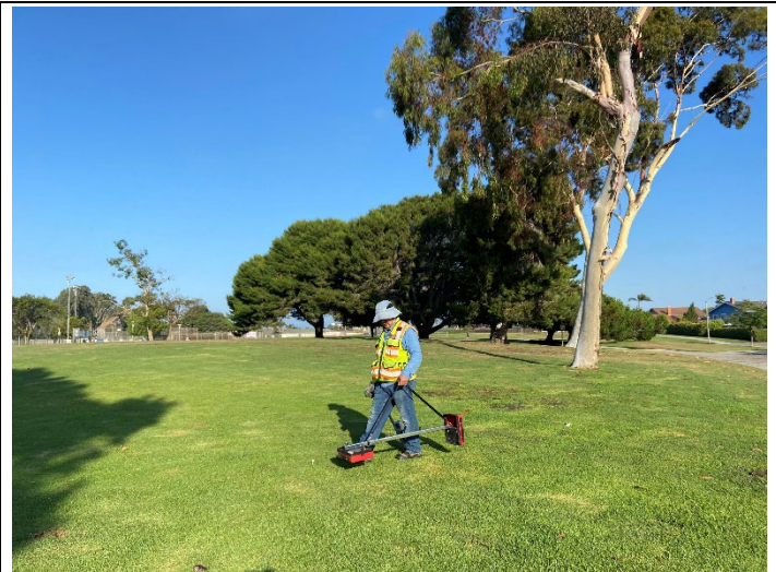
Geophysical survey being performed using the Fisher metal detector around the Oil Well #2 area.
