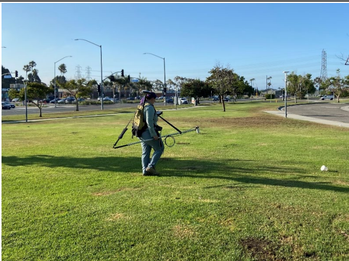
Geophysical survey being performed using the magnetometer at Oil Well #1 location (looking south)
