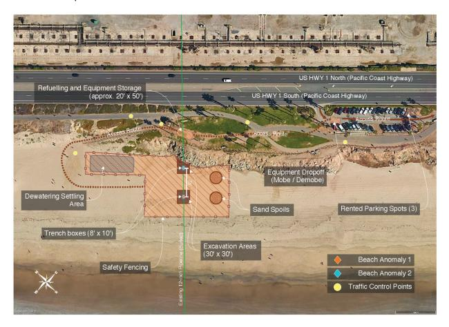
Dewatering of the excavations may be required; in which case the water will be discharged into a permitted settling basin that will be dug adjacent to the work area. Alternatively, divers will access the repair sites and work in the submerged excavation.
